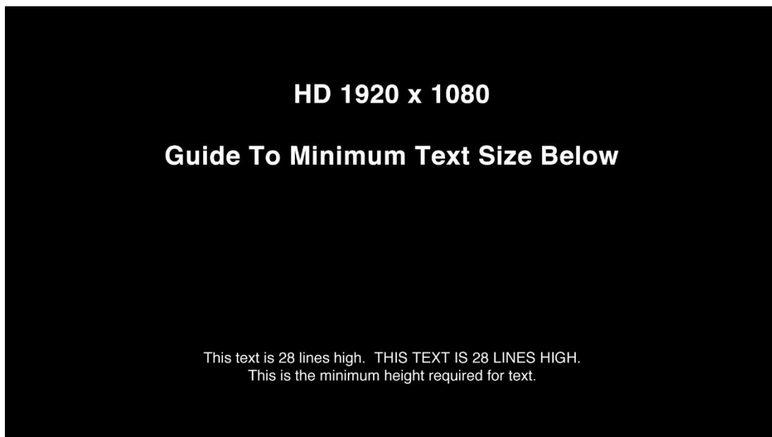
Figure B.12 Minimum height for text in a High Definition Television Commercial
